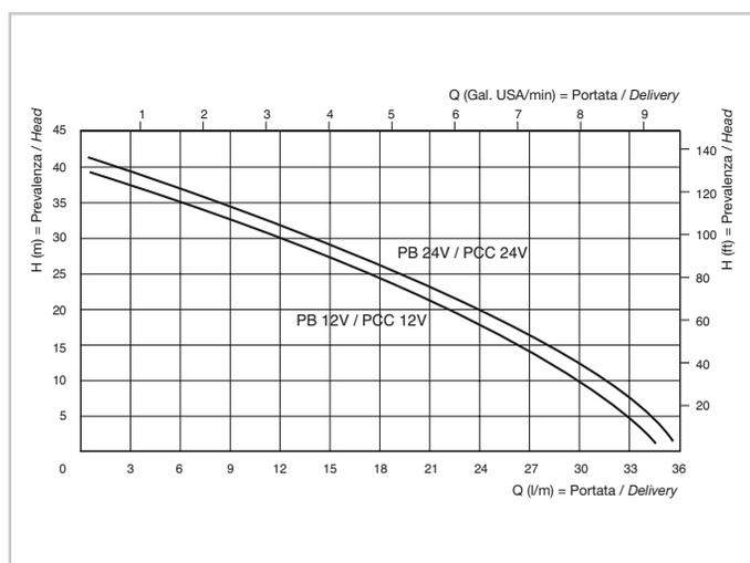
Peripheral pumps suitable for developing high pressures at limited deliveries. The pump casing is available in cast iron for fresh water or gas oil (PCC), or in bronze for sea water (PB).
